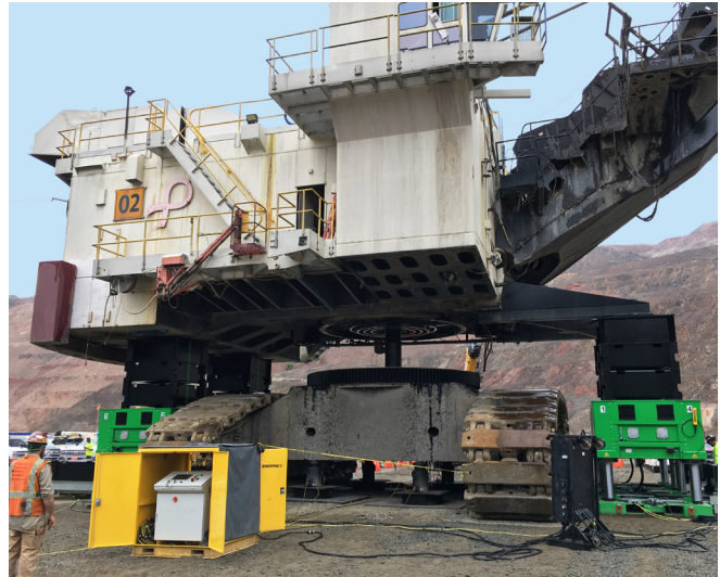
Alignment is checked very closely to ensure lifting under the correct parts and that no damage will take place.
