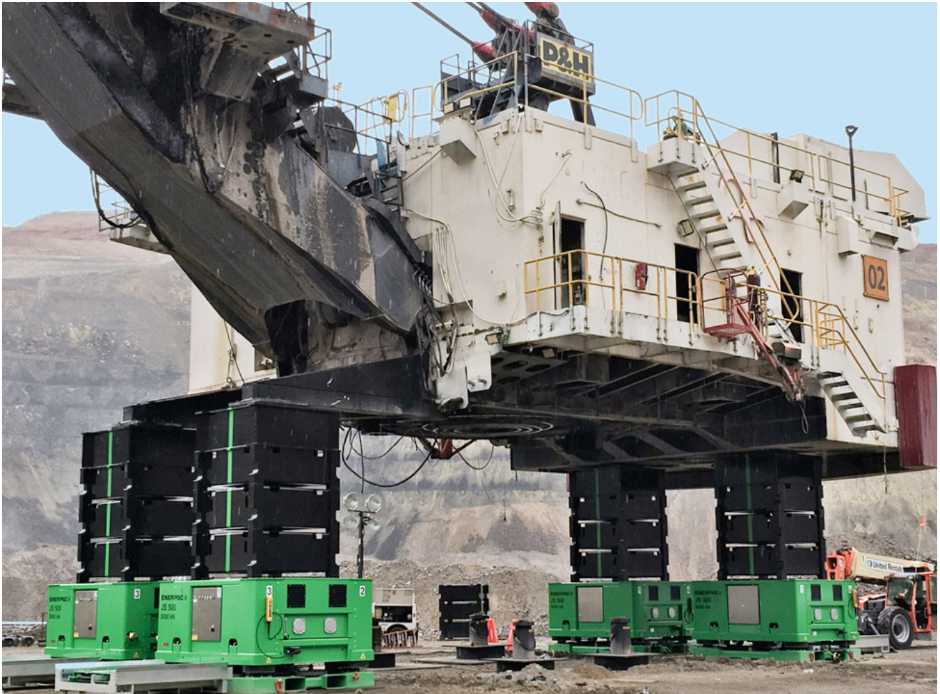
The JS 500 Jack-up system has a lifting capacity of 2,000 metric tons.
