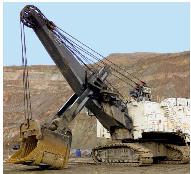
The rope shovel was moved to the maintenance area to remove the dipper sticks, bucket and any unnecessary weights that do not need to be lifted and then returned to the pad to perform the lift.
