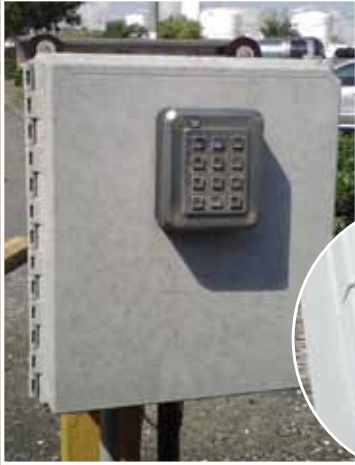
Prolonged UV exposure can cause fiberbloom on fiberglass enclosures, a form of surface degradation that results in loss of color and gloss.
