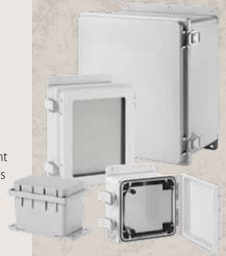
Hybrid PC polyester blend enclosures offer a wide range of benefits, including excellent impact resistance. Since they do not contain glass, these enclosures are not susceptible to fiberbloom.
